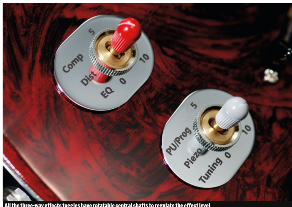
All the three-way effects toggles have rotatable central shafts to regulate the effect level
