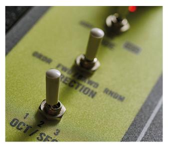
stored in memory (retained between power cycles). It's strictly a step sequencer no real time recording with notes entered from the keyboard itself. Rests, ties, and accents are entered using the three buttons above the pitch and mode wheels. Recorded sequences can be latched and transposed on the fly by pressing any key. The toggle switch used for selecting the arpeggiator's octave is also used to select which of the three stored sequences is played.
