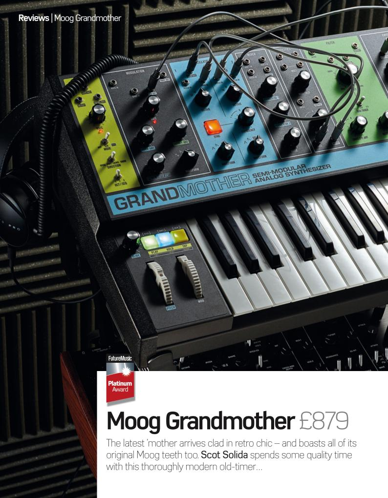
CONTACT who: Moog Music / Source Distribution web: www.sourcedistribution.co.uk KEY FEATURES Monophonic semi-modular analogue synthesiser with 32-note, velocity-sensitive Fatar keyboard, sequencer and arpeggiator. 41 patch points with 21 inputs, 16 outputs and a Parallel-Wired 4-jack Mult. External audio input. Spring reverb
