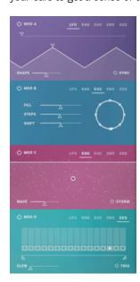
modulation signal. EUC, a Euclidean Sequence Generator, creates gate signals based on a shifting pattern of beats determined by the fill, steps and shift parameters. The beauty of this form of pulse generator is that it responds well to random tweaking, yet produces musically useful results. The final two modulators, ENV and SEQ, return to more conventional territory with an ADSR envelope and tempo-locked level/ gate sequencer.
