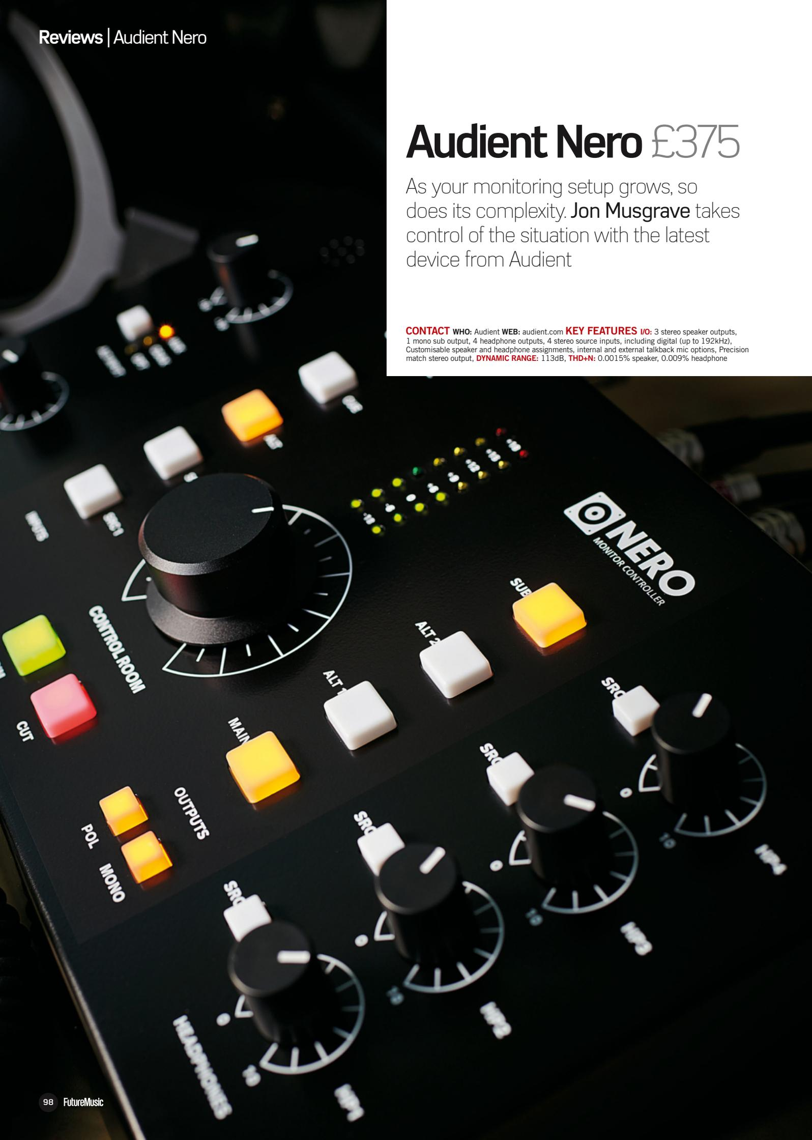
**N**ero is a high fidelity desktop format monitor controller from Audient, designed to act as the final communication device between your DAW, monitors and anyone you're recording.
