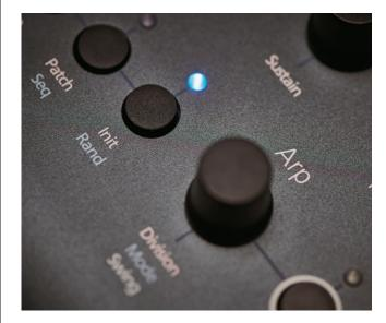
instant beat repeat effect. Sequence steps are handily shown by the lights across the panel. Finally, the 32-step arpeggiator is fully programmable and transposable with plenty of direction modes, time divisions and swing. Both the arp and sequencer sync to MIDI and the arp can accept external MIDI input too. See also the Modal app (Windows/Mac/ iOS/Android/VST/AU) for editing sequence info if you prefer.
